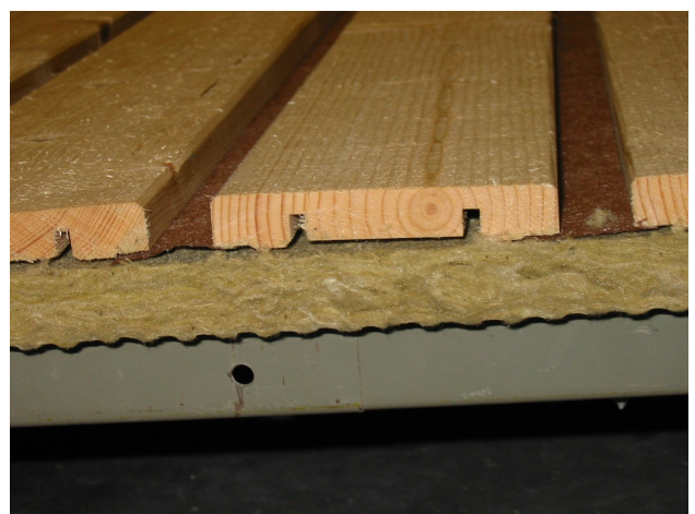
3: detail variant 2 (with mineral wool)
